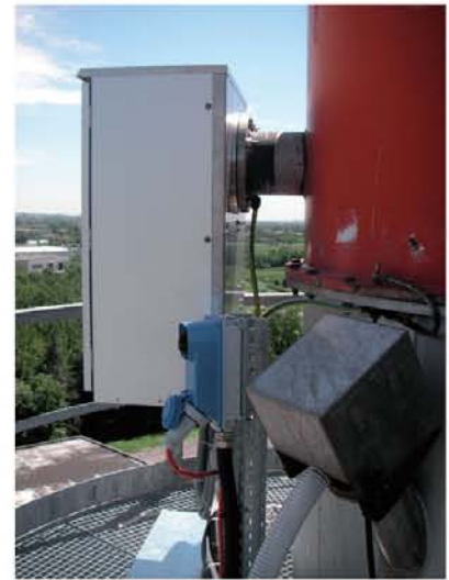
DECS sampling unit and EN1948 test equipment (TCR Tecora Isostack) during parallel sampling
