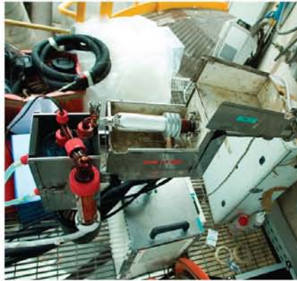
DECS sampling unit and EN1948 test equipment (TCR Tecora Isostack) during parallel sampling
