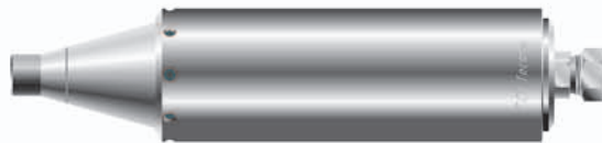
Assembled Impactor with nozzle and cone for sampling in vertical position
